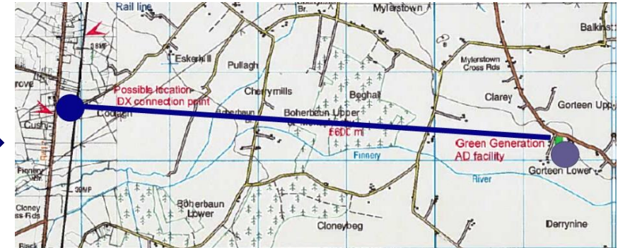
~ 5 km low pressure biogas pipeline
