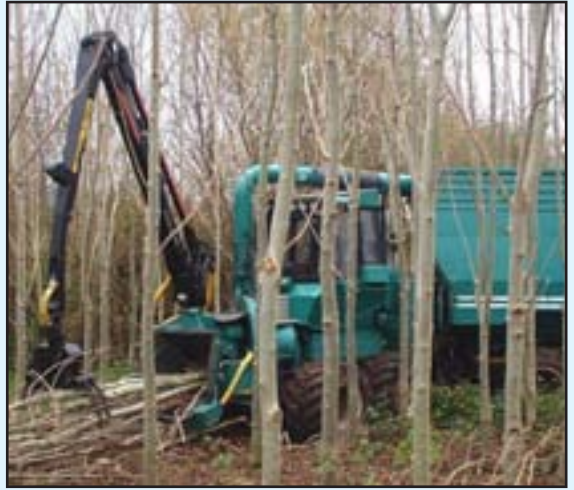
Terrain chipper producing energy wood
