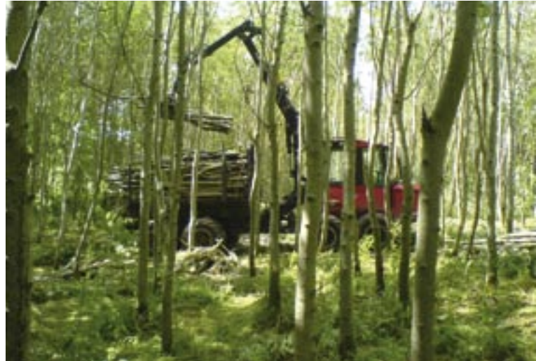
Figure 10. Extraction of broadleaf thinnings by a forwarder
