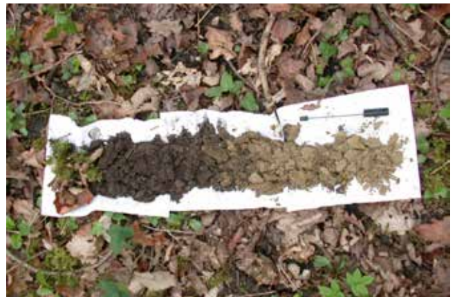
Figure 3 A soil profile derived with a Dutch soil auger. Samples are taken from the same core site and laid out in sequence (i.e. topsoil above subsoil above parent material) to ascertain the soil type.
