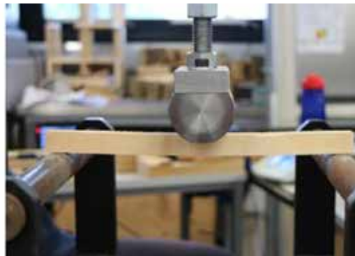
Figure 7: Testing timber quality of Sitka spruce families using a TreeSonic™ (left) which measures time of flight between two probes and has been linked to bending strength of timber (middle photo) and ring width analysis using the WinDENDROM™ system.
