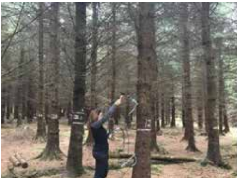
Figure 7: Testing timber quality of Sitka spruce families using a TreeSonic™ (left) which measures time of flight between two probes and has been linked to bending strength of timber (middle photo) and ring width analysis using the WinDENDROM™ system.
