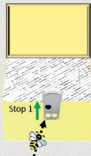
When bee lock is at 'Stop 1' position, bees can enter colony.
