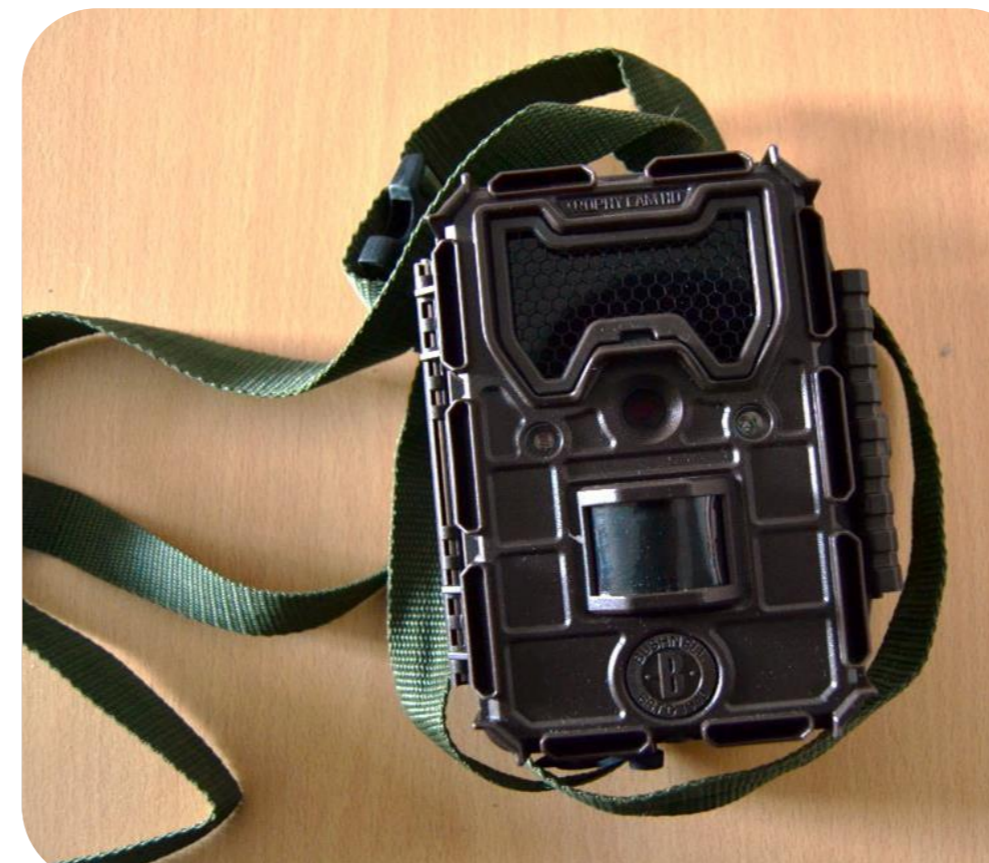
Fig 5 – High resolution hydrometric station of the Agricultural Catchments Programme (Teagasc) at the Ballycanew catchment; Fig.6 – Motion-activated infrared camera to be used in this study.
