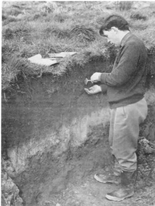
Plate 4—Soil profiles representative of each soil series are examined and described. The various horizons are sampled for laboratory analyses.
