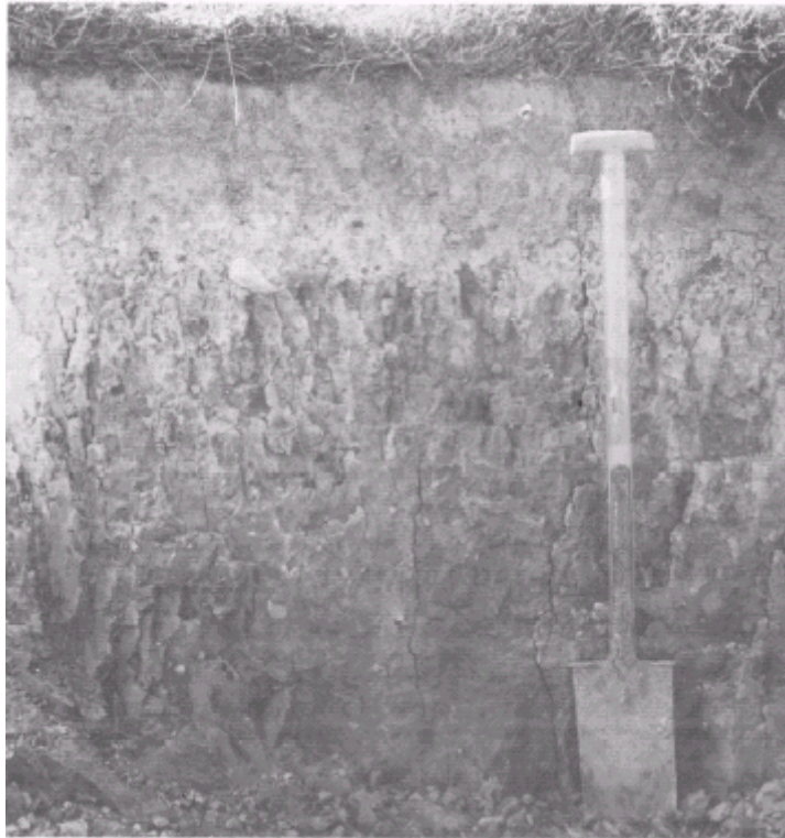
Plate 18: Profiles of the poorly-drained Gley soils of Association 42 display a massive or weak coarse prismatic structure as well as a grey leached A2 horizon overlying a Btg horizon in which there is a significant increase in clay content.
