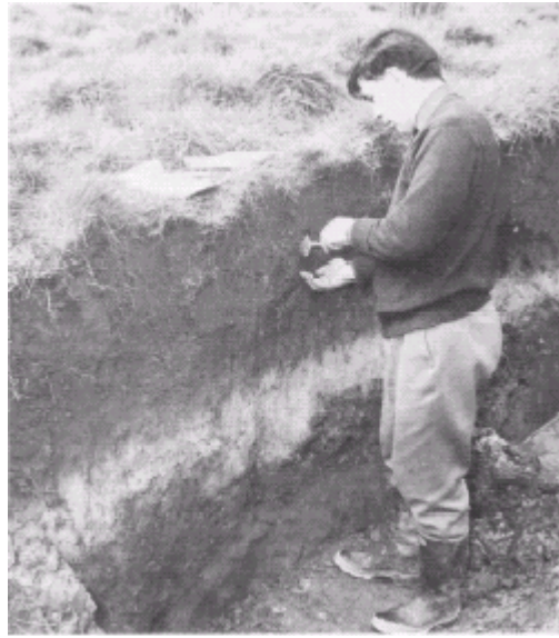
Plate 3: Soil profiles, showing a succession of different layers or horizons are examined, described and sampled for analysis.
