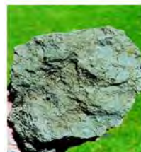
Poor: No visible macropores, massive structureless smooth surfaced, sharp edges
