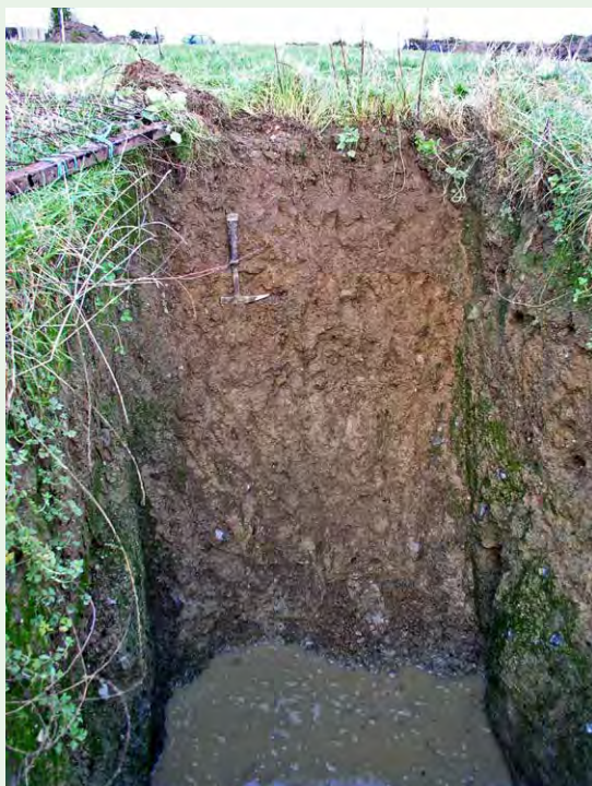
Figure 3. Permeable layers will be indicated by seepage of water into the soil test pit.
