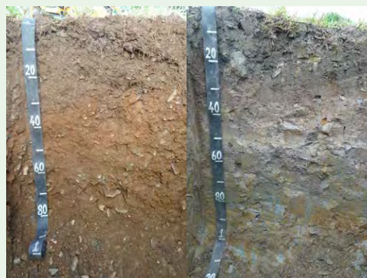
Figure 3. Soil (a) on the left is well drained, soil (b) on the right is poorly drained.
