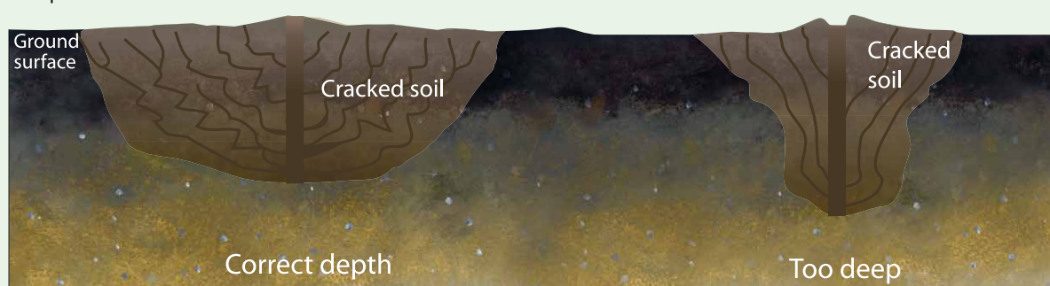
Figure 10. Effect of depth on the impact of subsoiling.
