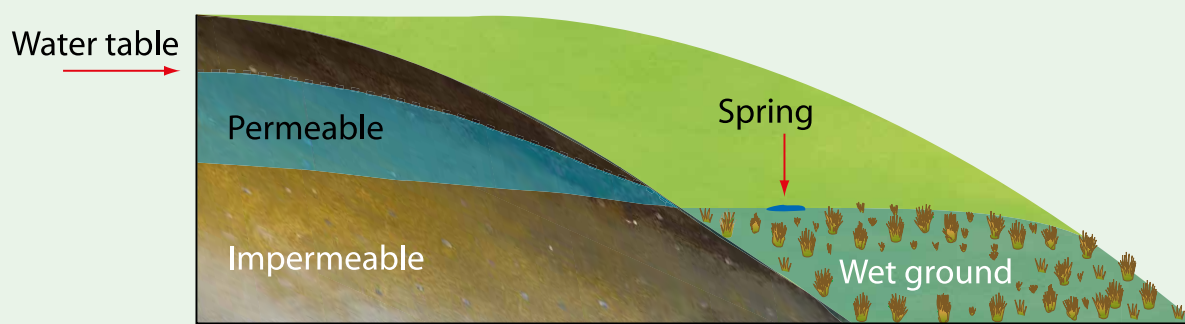
Figure 8. Cutaway of how an impermeable layer can result in springs emerging on a hillside (see also Chapter 1).
