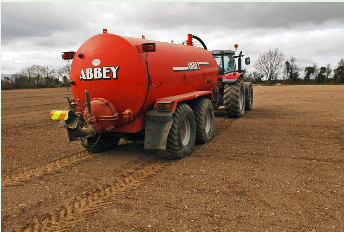
Figure 2. Different axle configurations can help distribute the load on the soil, but the tyres must be large enough to reduce ground pressure.
