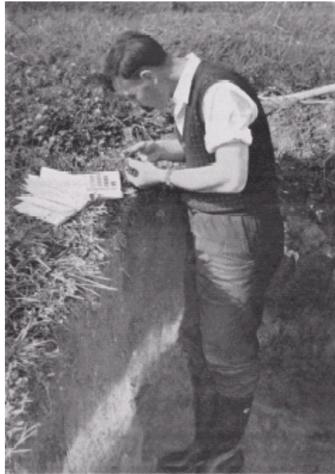
Plate 6—Soil profiles representative of each soil series are examined and described. Samples are taken from each horizon for laboratory analysis
