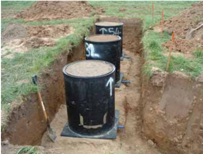
Johnstown Castle boasts a world-class field lysimeter laboratory, which allows us to continuously measure nutrient uptake, and losses to water and air from three contrasting soil types.
