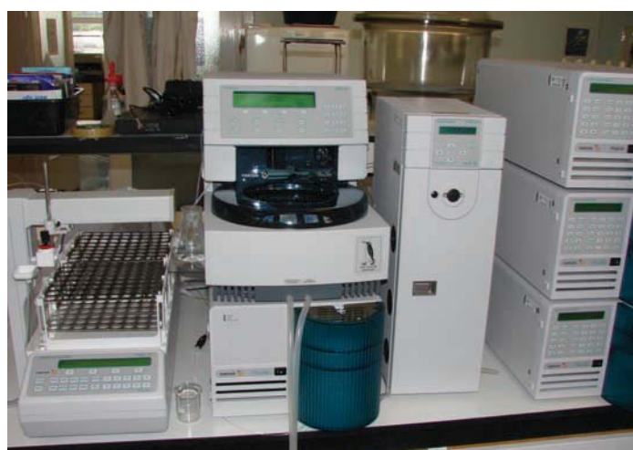
FIGURE 3: HPLC system with fraction collector and photodiode array detector at AFRC.
