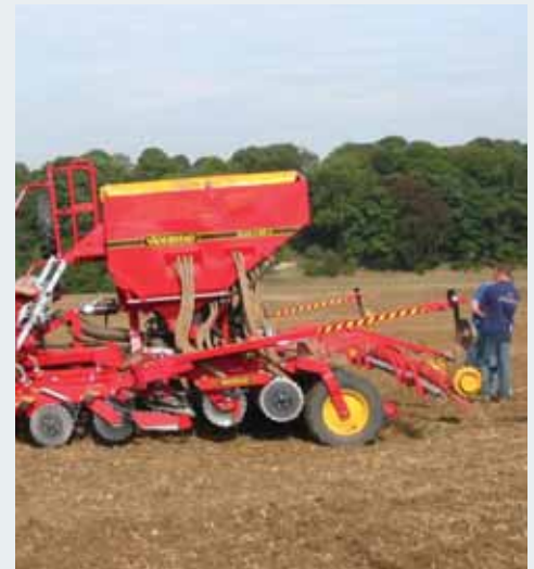
Seeder suitable for sowing into minimum-till ground.
