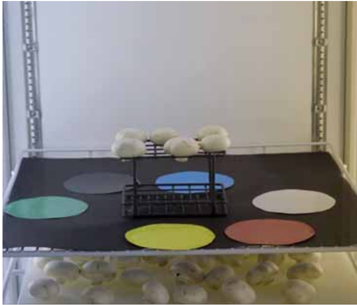
FIGURE 2: Image analysis set-up at DIT to observe whiteness reduction and the appearance of browning. The system is inserted inside an incubator with temperature and RH control.
