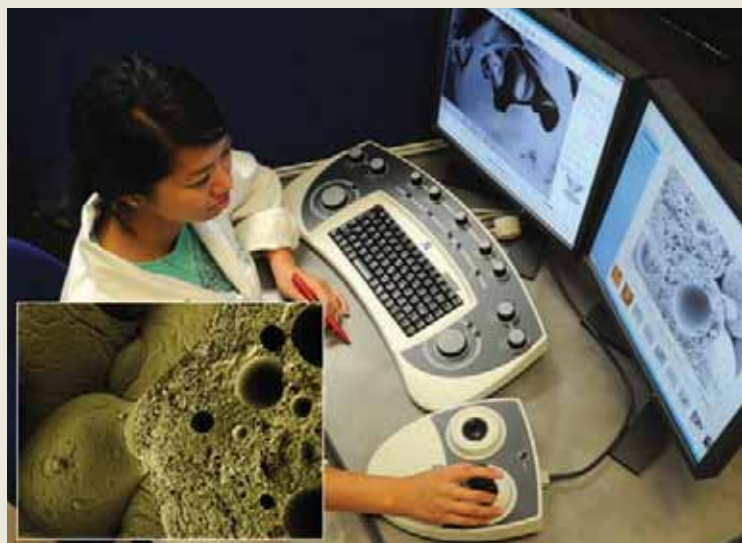
Figure 1: Teagasc research officer Vivian Gee operating the new scanning electron microscope. Inset is an image of a fractured milk powder particle to show surface detail and internal aerated structure.
