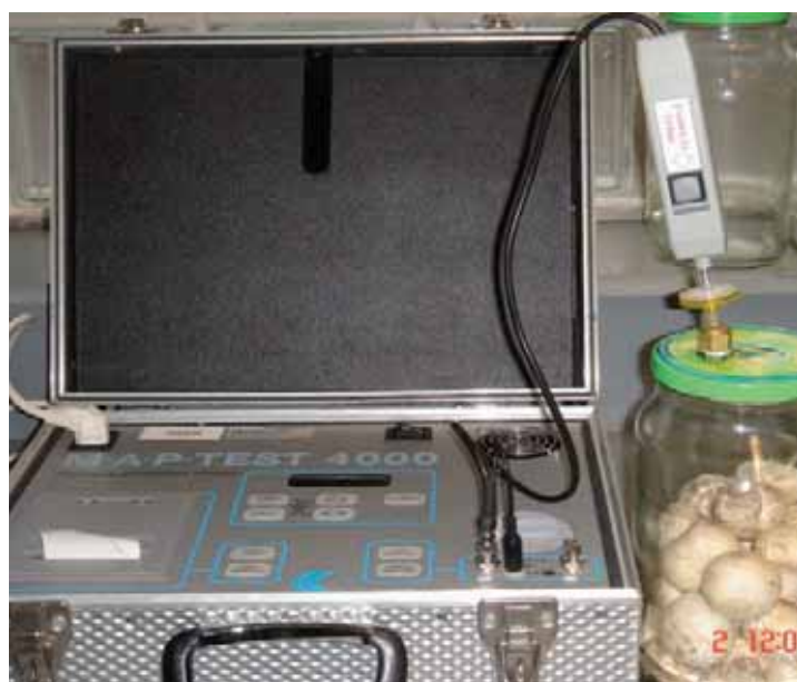
Figure 4. Closed system respirator with an O 2 and CO 2 analyser.
