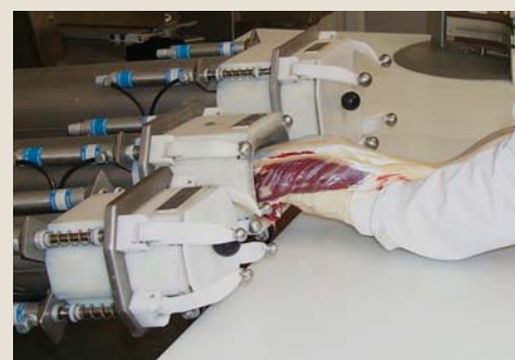
Striploin being inserted into Pi-Vac® packaging system. A novel early post-mortem technique that may alleviate the toughening effect of hot-boning.
