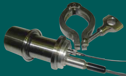
FIGURE 2: Light backscatter syneresis sensor design and optical configuration used for monitoring coagulation and syneresis to improve control of curd moisture content.
