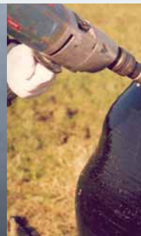
Core sampling a bale using a sterilised mechanical bit.
