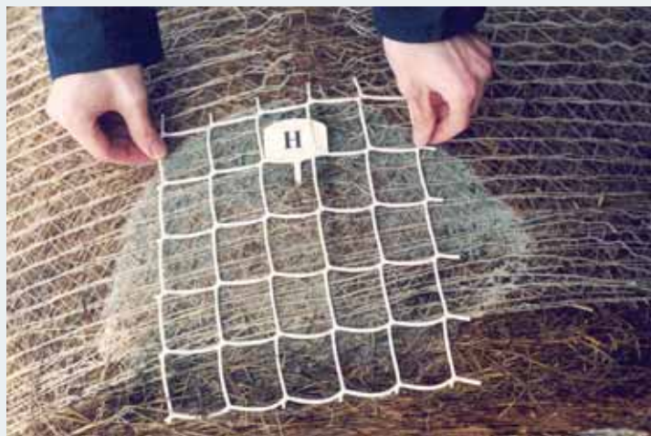
Measuring the area of Penicillium roqueforti growth on the surface of a bale.
