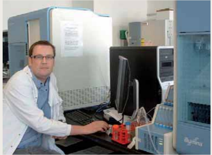
An Illumina Next Generation Sequencer has recently been purchased by Teagasc to analyse the DNA and RNA sequences from disease-resistant and susceptible animals.
