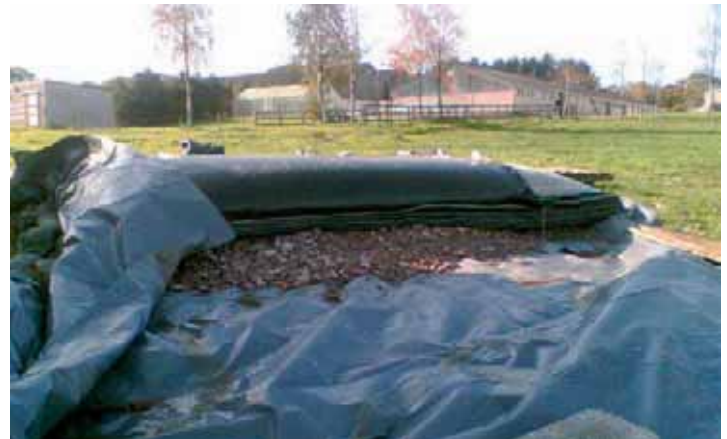
Clear liquid seeps from a Geotube filled with pig manure at Moorepark.
