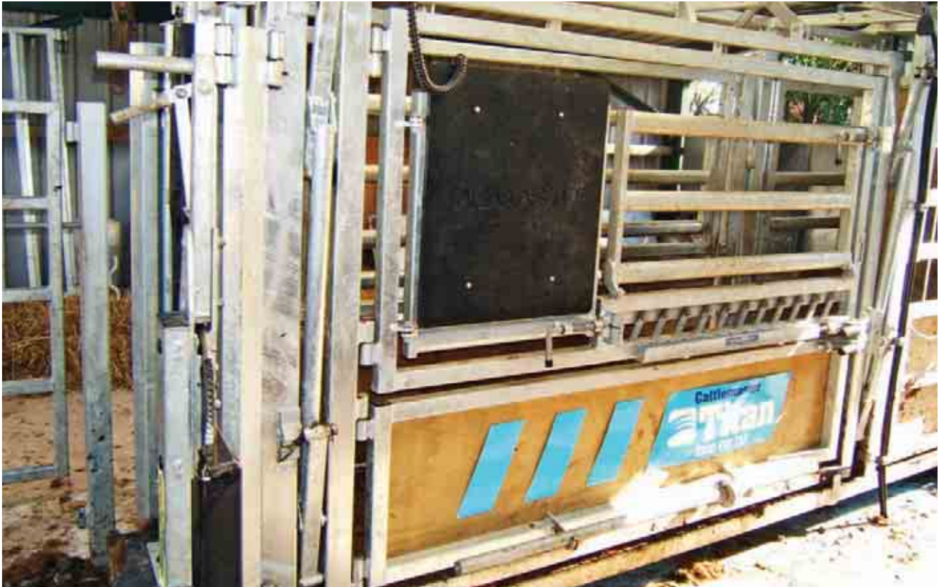
An automatic squeeze crush fitted with an EID scanning board reads an animal's electronic tag and weighs it at the same time on Robert Neill's farm.
