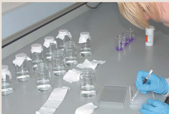
FIGURE 1: Preparing samples for ^{15}\text{N} analysis.
