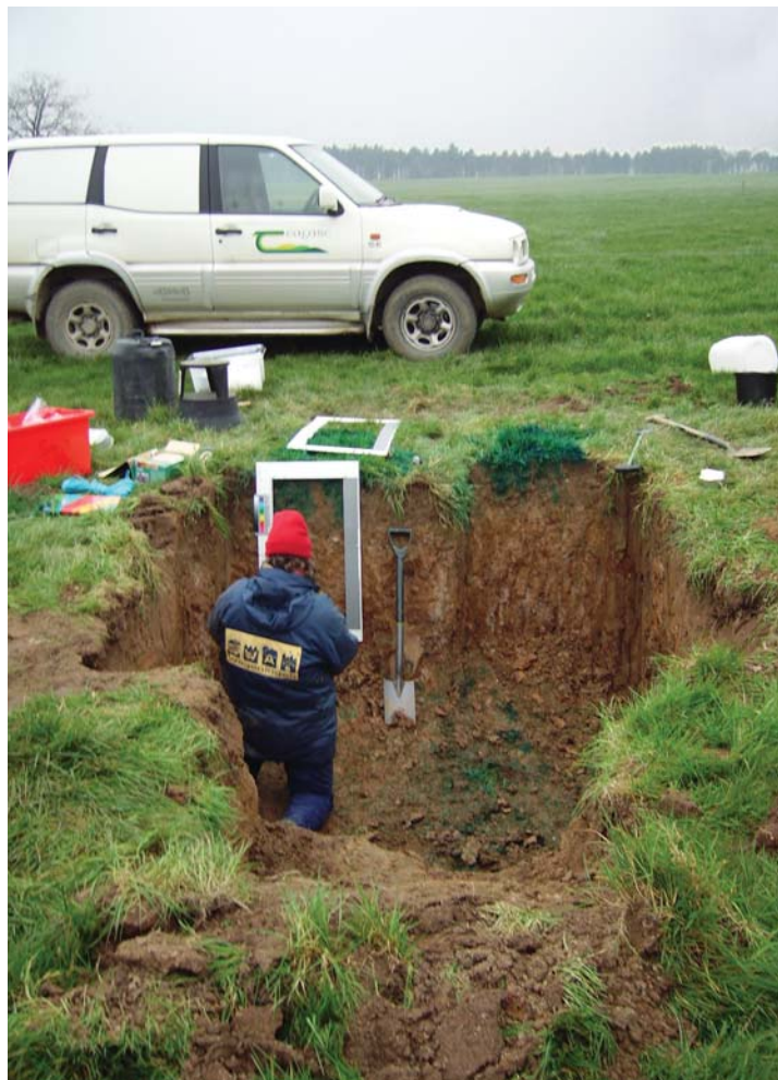
Tracing pathogen transport pathways in soil using blue dye at field sites.
