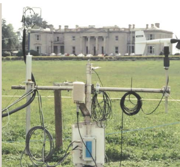
TOP LEFT: Collars to measure methane from cows. BOTTOM LEFT: Static chambers for nitrous oxide measurement. LEFT: Field-scale CO 2 quantified by eddy covariance.
