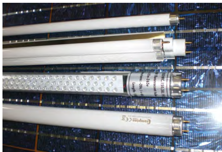
FIGURE 2: Types of lighting available for milking parlours (from top): T5 tube; T8 to T5 converter; LED tube; and, conventional T8 tube.
