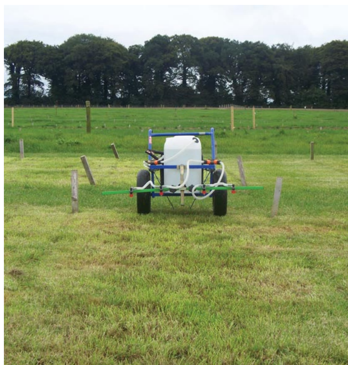
FIGURE 2: Sprayer to apply DCD as a fine particle suspension to grass plots.
