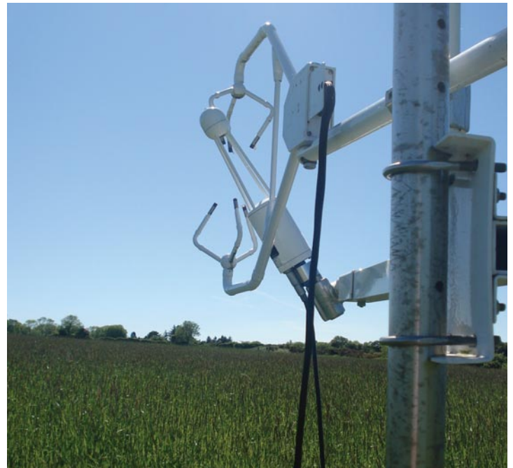
Eddy covariance tower measuring field-scale CO 2 fluxes over a reed canary grass stand at Johnstown Castle.
