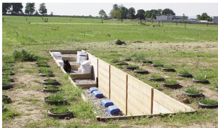
Lysimeters installed at Teagasc, Moorepark, to monitor nutrient leaching and N_2O emissions.
