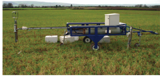
Eddy covariance system for field CO 2 measurement
