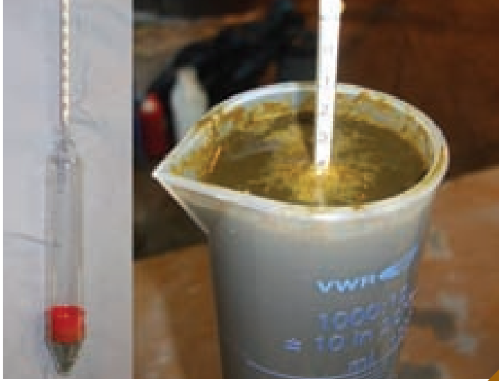
Figure 1: Slurry hydrometer with graduated scale used to estimate the slurry dry matter concentration in a well-mixed slurry sample.
