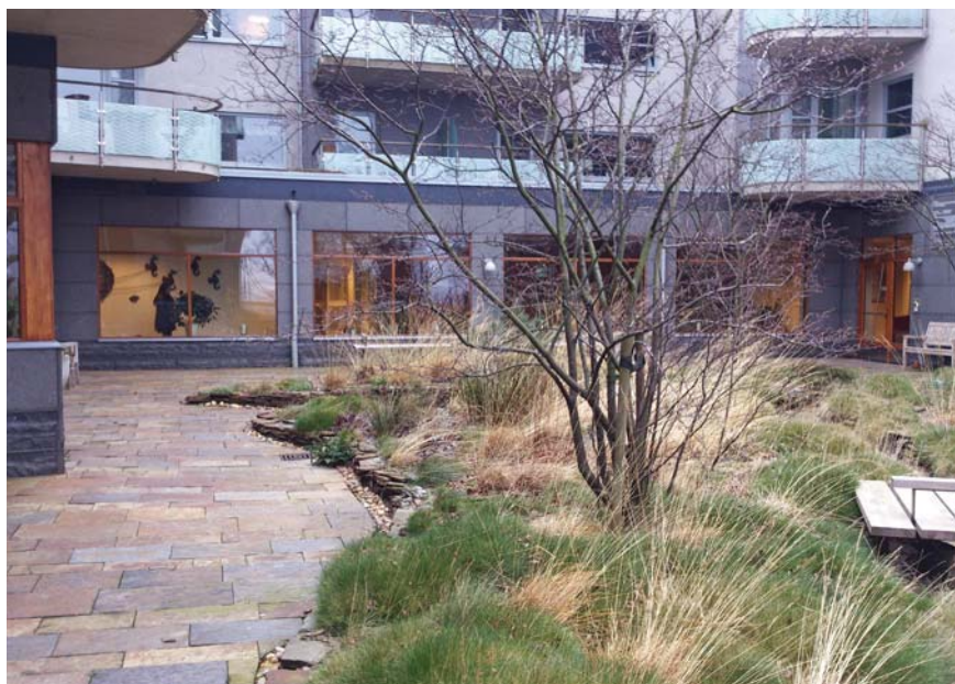
Award-winning apartments in Malmo, Sweden, use rain gardens in courtyards to drain water from hard surfaces.
