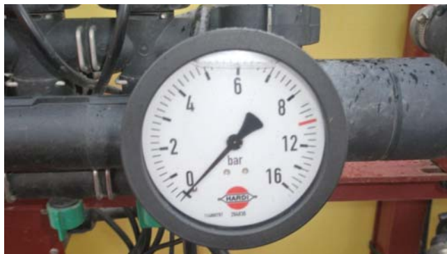
The pressure gauge must be accurate, be easily readable from the driver's seat and have scale markings of at least every 0.2-bar up to five-bar.
