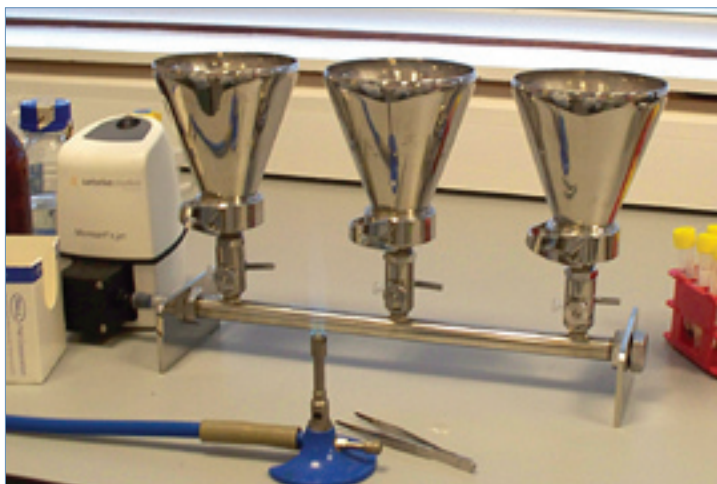
Filtration apparatus used for extraction of E. coli from soil and sewage sludge.
