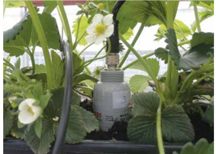
SM 150 moisture sensor in situ in growing trough.
