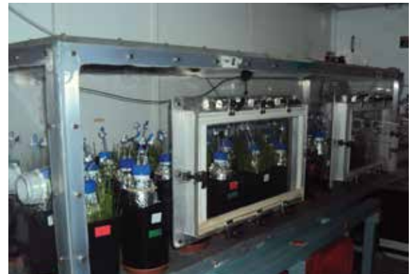
Steady-state isotope labelling chamber: ^{13}\text{C} -labelled \text{CO}_2 at ambient concentrations is passed through the chamber over the growth period of the plant. Use of stable isotopes allows for differentiation between photo-assimilated C and soil-derived C in total \text{CO}_2 efflux to quantitatively measure plant-C inputs and soil-C outputs.
