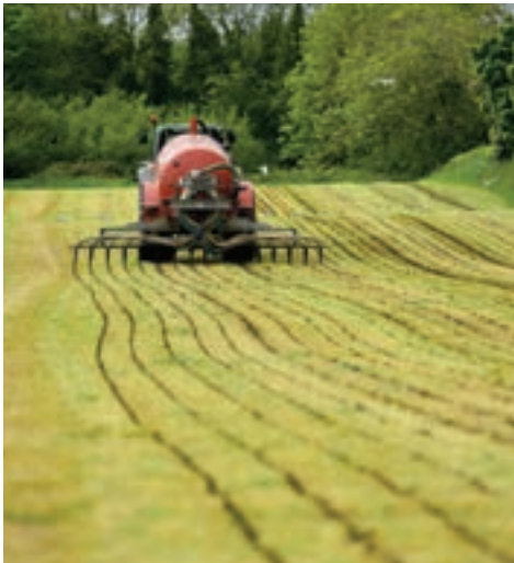
Trailing-shoe slurry spreading.
