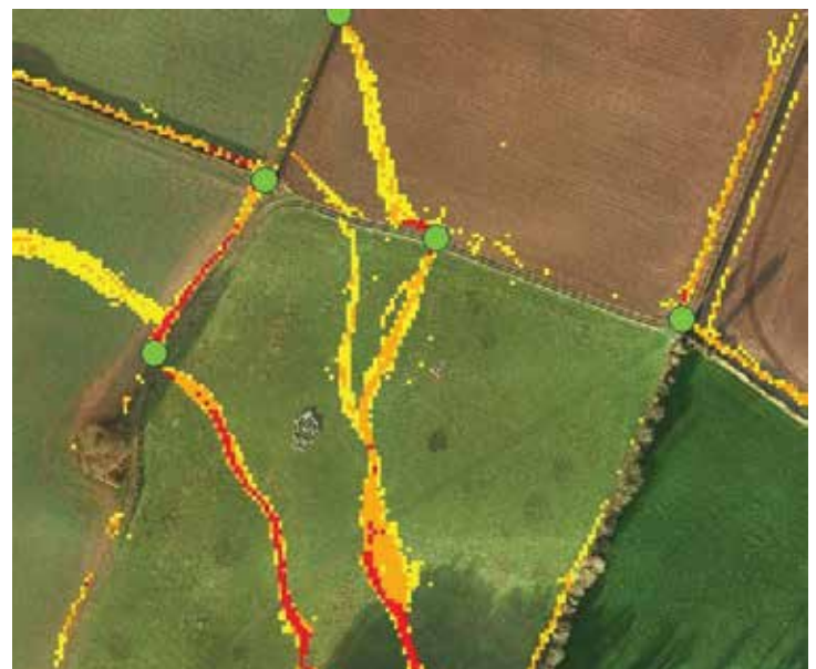
Figure 3. HSA map showing runoff pathways generated during small (red), medium (orange) and large (yellow) rainfall events. Also indicated are breakthrough points at field boundaries (green dots) and a delivery point (blue dot) at the stream (grey line) where mitigation measures should be targeted.
