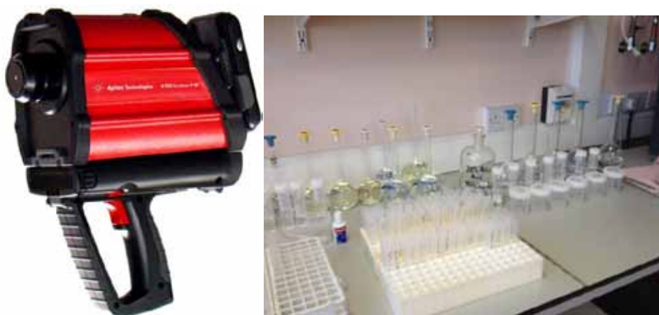
Figure 2. Portable soil spectrometers (left) for measuring multiple soil properties in one scan as an alternative to wet chemical tests (right) that are often sensitive to soil properties.
