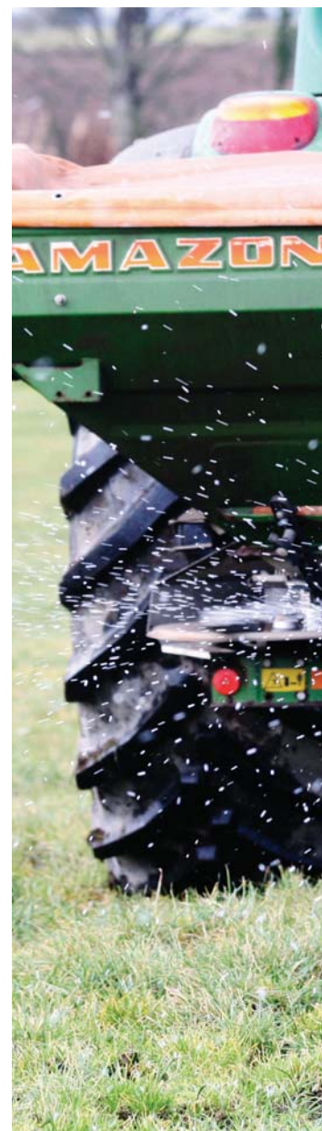
Fertiliser spreaders will differ in their ability to spread evenly, so it is very important to look at spread patterns from independent sources and choose bout widths carefully.
