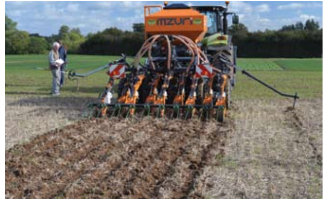
Strip tillage drill sowing directly in stubble .
