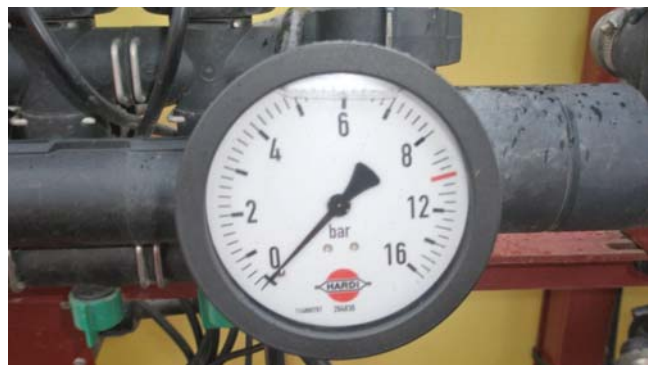
The pressure gauge must be accurate, be easily readable from the driver's seat and have scale markings of at least every 0.2-bar up to five-bar.
