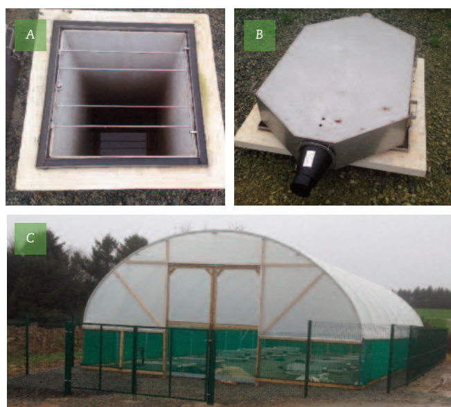
FIGURE 2: New slurry storage facility at Teagasc Johnstown Castle showing: (a) one of twelve 1m 3 concrete storage tanks; (b) dynamic chamber used to measure ammonia and greenhouse gas emissions; and, (c) overview of the facility.
