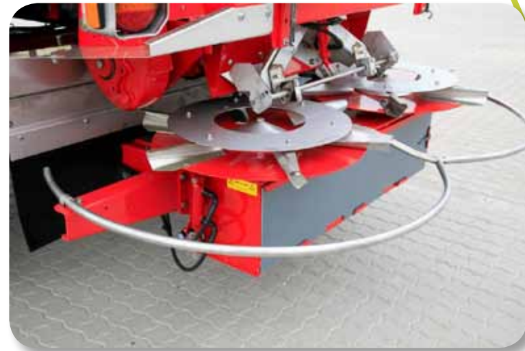
Figure 1:- Fertiliser spreader developments have been mainly confined to twin-disc units over the last number of decades.
