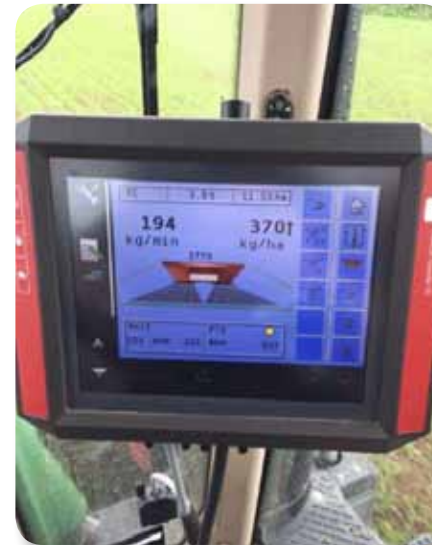
Figure 12:- In cab controls to change fertilizer spreader application rates
