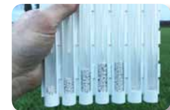
Figure 8:- Fertiliser spread pattern where boundary mechanism not in place
