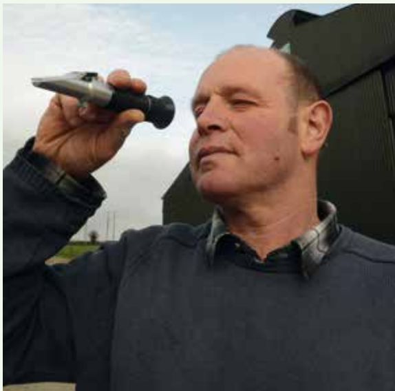
A Brix refractometer is used to indirectly evaluate the level of immunoglobulins in colostrum.
