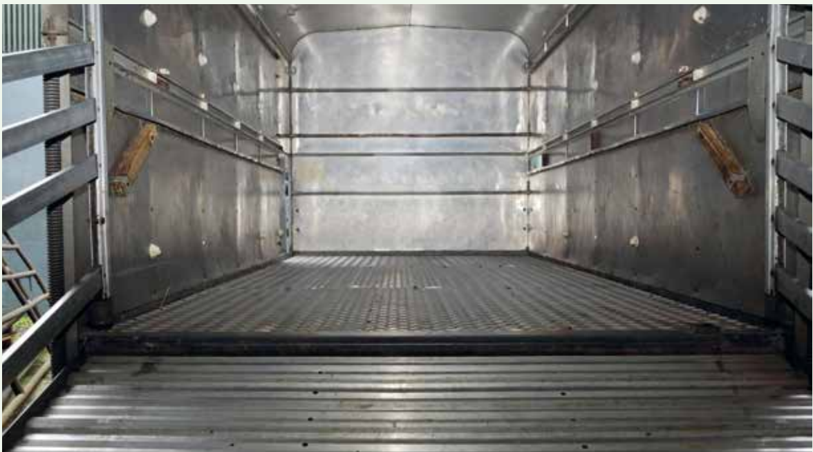
A non-slip unloading ramp will help prevent calf injury.
