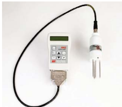
Figure 3: Soil moisture probe.
