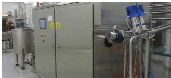
FIGURE 1: Microwave volumetric heating system being assessed in the SACCP ( http://www.advancedmicrowavetechnologies.com/equipment/ ).
