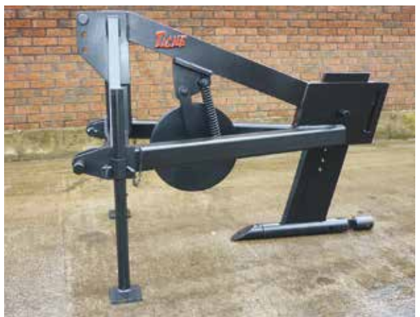
Mole plough showing cylindrical foot and expander
