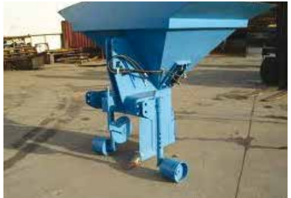
Gravel Mole plough showing hopper
