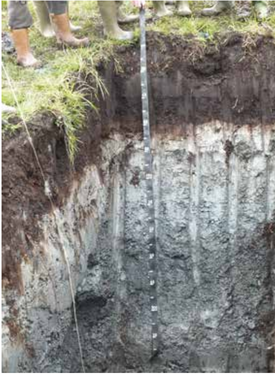
Test pit excavation
