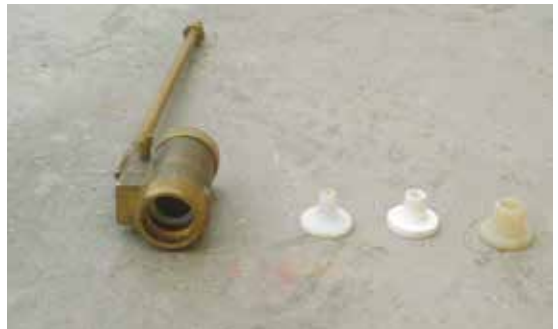
This is a bulkier version of the \frac{1}{2} inch ballcock, in which fits the low pressure jet as well. Note the bigger seating gasket for the jet inside.
