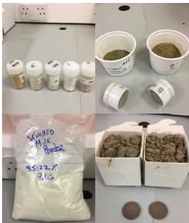
The range of agri-food samples currently being analysed using XRF: biosolids and dairy waste; grass; soil; and, milk powder.
