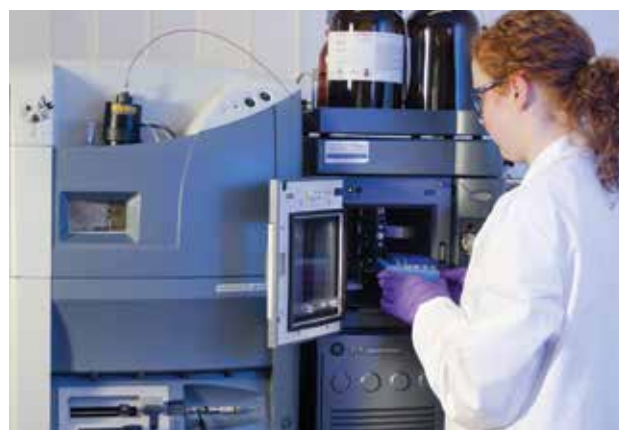
Figure 1: Analyst placing sample extracts for injection into liquid chromatograph for LC-MS/MS analysis
