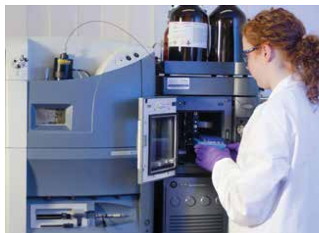
Figure 1: Analyst placing sample extracts for injection into liquid chromatograph for LC-MS/MS analysis
