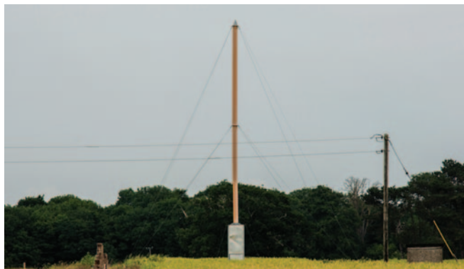
FIGURE 1: A 12.2m high insect suction tower, which passively samples the passing air for flying insects such as aphids.
