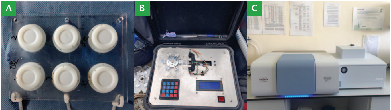
FIGURE 1 (from left): passive samplers deployment rig (A) and lab-on-a-disk (B) for in-situ nutrient analysis, both developed at the DCU Water Institute. (C) Bruker FTIR spectrometer used at Teagasc Johnstown Castle to scan soils.
