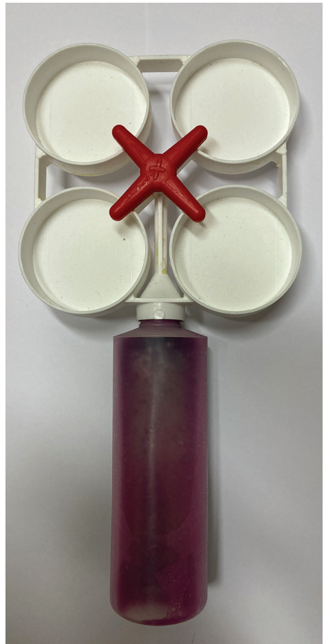
CMT paddle kit – test cows five days after calving to identify high-SCC quarters.
