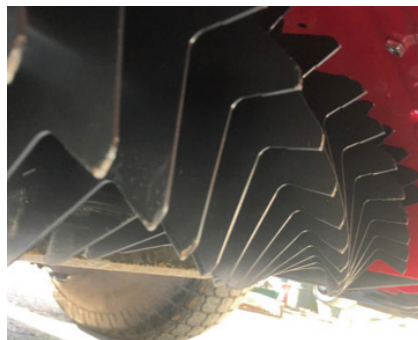
Using verticutting blades on a scarifier.
